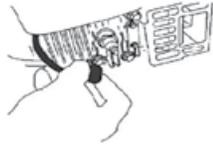
3. After performing the maintenance procedure(s), connect the spark-plug wire to the spark plug.
