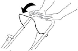
**⚠ Important:** When releasing the blade control bar both the blade and engine should stop within 3 seconds. If they both do not stop properly discontinue use of the machine and contact an authorized Service
