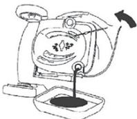
4. After drain the used oil, return the machine to the normal operating position.
