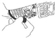
3. After performing the maintenance procedure(s), connect the spark-plug wire to the spark plug. Important: Before tipping the machine to change the oil or replace the blade, allow the fuel tank to run dry through normal usage. If you must tip the machine prior to running out of fuel, use a hand fuel pump to remove the fuel. Always tip the machine onto its side with the dipstick down.
